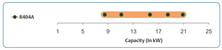
Note: The above capacity data are at the following condition. Ambient Temp. +38°C, Evaporating Temp. - 25°C, Return Gas Temp. +18.3°C, Subcooling 2.8K
